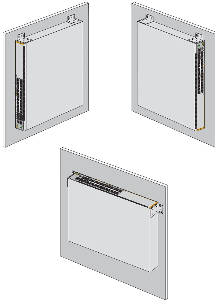
Figure 42. Positioning the x530-28GTXm or x530-28GSX Switch on the Wall
