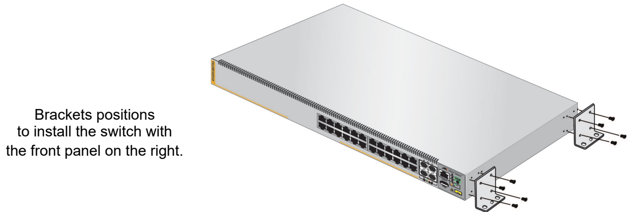
Figure 46. Installing Two Brackets on the x530-28GTXm or x530-28GSX Switch
