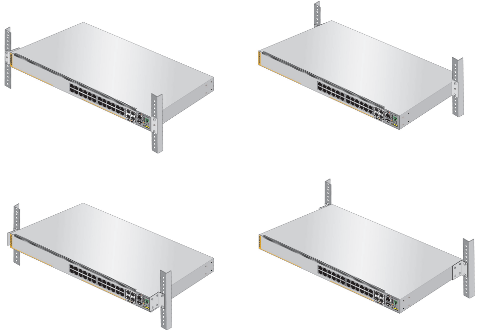
Figure 39. Switch Orientations in an Equipment Rack
